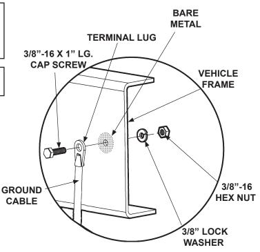
BOLTING GROUND CABLE TO VEHICLE FRAME FIG. 33-2
